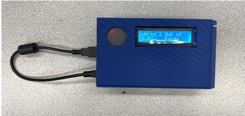
Figure 3.2- Assembled Battery Operated AS7265X Irradiance meter
