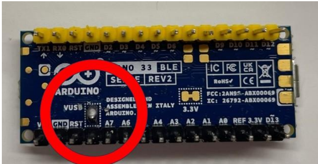
Figure 2.9 - 5V pin activated.
