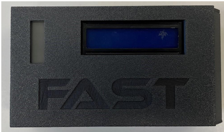
Figure 1.10- Completed Irradiance Meter with APDS9960 Sensor.
