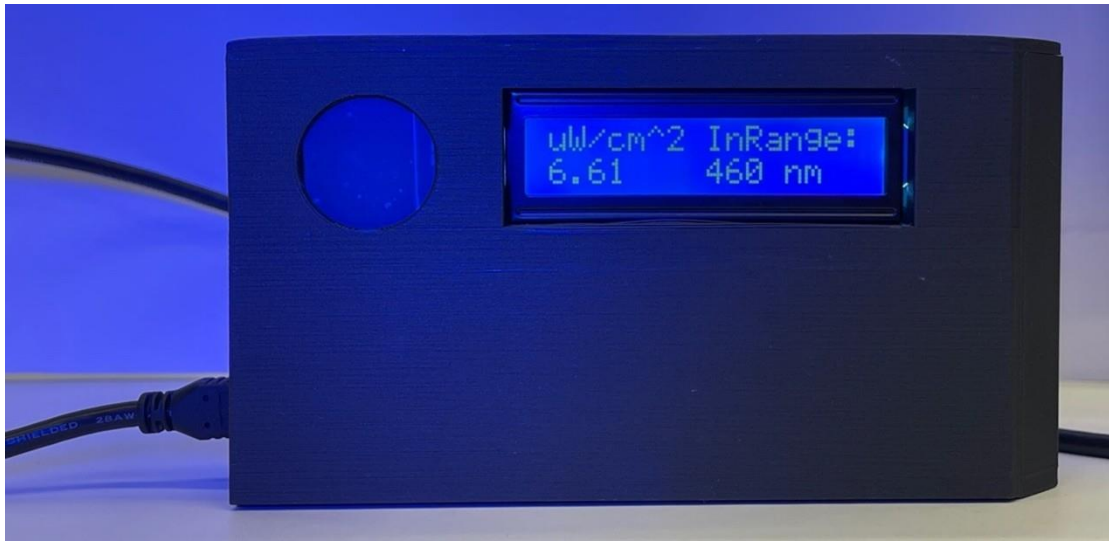
Figure 2.13- Irradiance Meter displaying calibrated results
