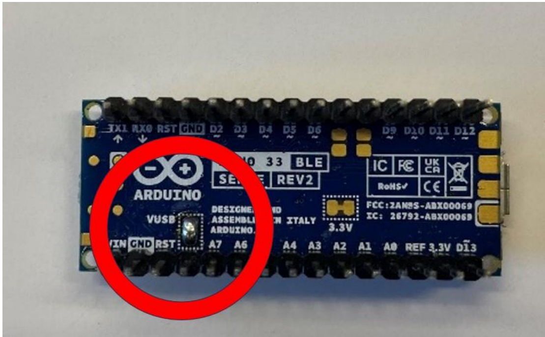
Figure 1.7- Soldered pads to access 5V.
