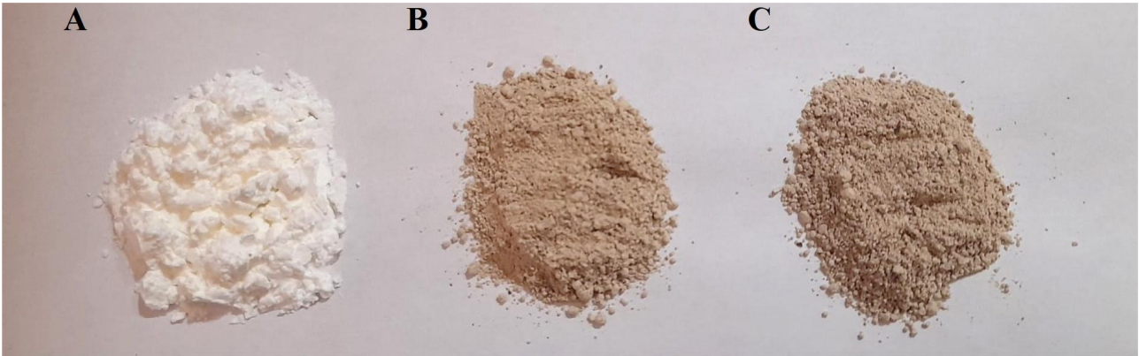
Figure 2. Photographic representation of the commercial starch (A), Q. robur starch extract by HP at 333 MPa for 17.4 min (B), and Q. robur starch extract by PEF using an electric field intensity of 0.1 kV/cm for 63.3 \mu s (C). HP: hydrostatic pressure; PEF: pulsed electric field
