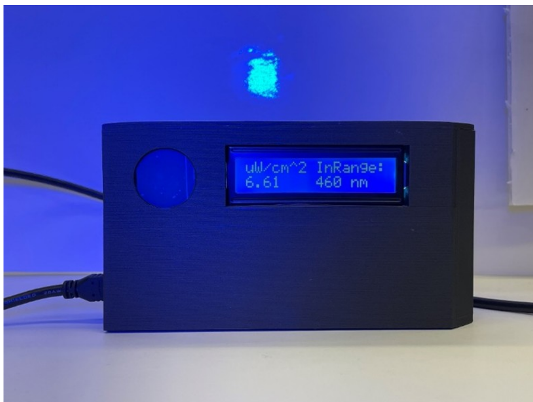
Figure 7. Open source irradiance meter displaying light source characteristics.
