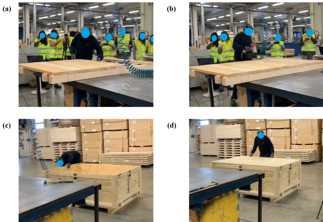
Figure 1. Wooden box workstation. (a) Placement of the wooden planks. (b) Operator using the nail gun. (c) Assembly of the container with a nail gun. (d) Closing the container with its lid.
